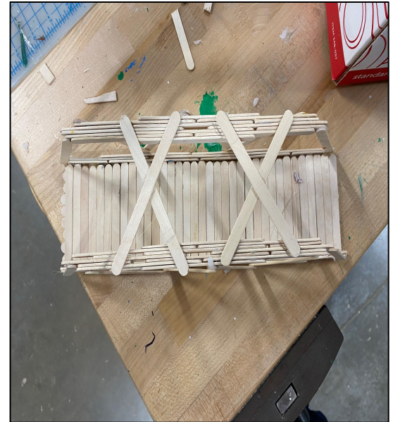
An x-bracing on the top of the bridge
